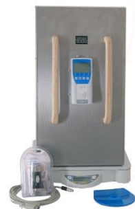
Figure 4: Example of a moisture meter to measure moisture content of wood chips. 6
