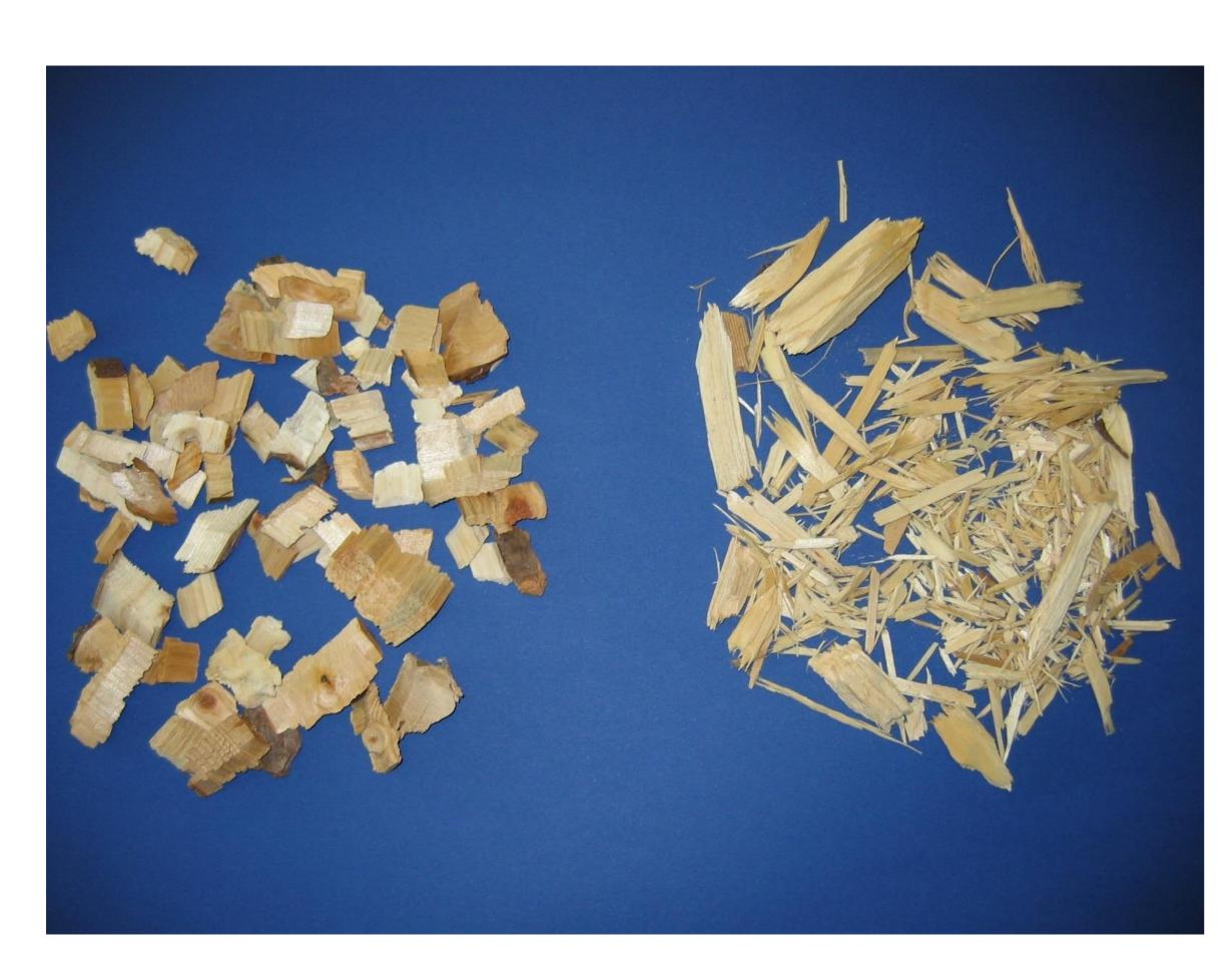
**Wood chips** (left) are defined as following: chipped woody biomass in the form of pieces with a defined particle size produced by mechanical treatment with sharp tools such as knives. Wood chips have a subrectangular shape with a typical length 5 to 50 mm and a low thickness compared to other dimensions. **Hog fuel** (right) is fuelwood in the form of pieces of varying size and shape, produced by crushing with blunt tools such as rollers, hammers, or flails.
